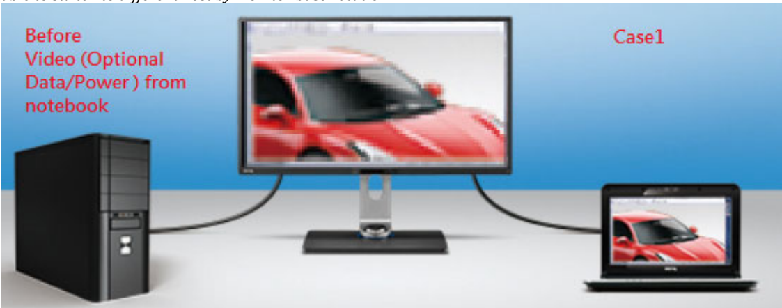
Figure 4. An example topology if using 2 of USB-C to connects to 2 of host system, by using angle sensor to let scalar know the angle change, also able to switch to different host by monitor base rotation.
