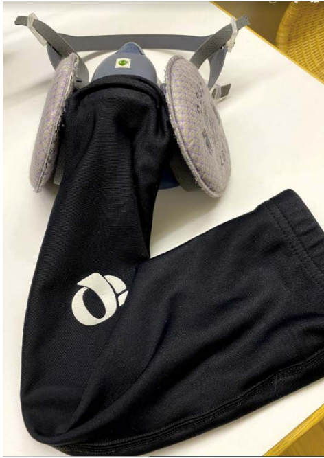
Mask with a flexible tube (woven sleeve) secured to mask outlet by Velcro tape
