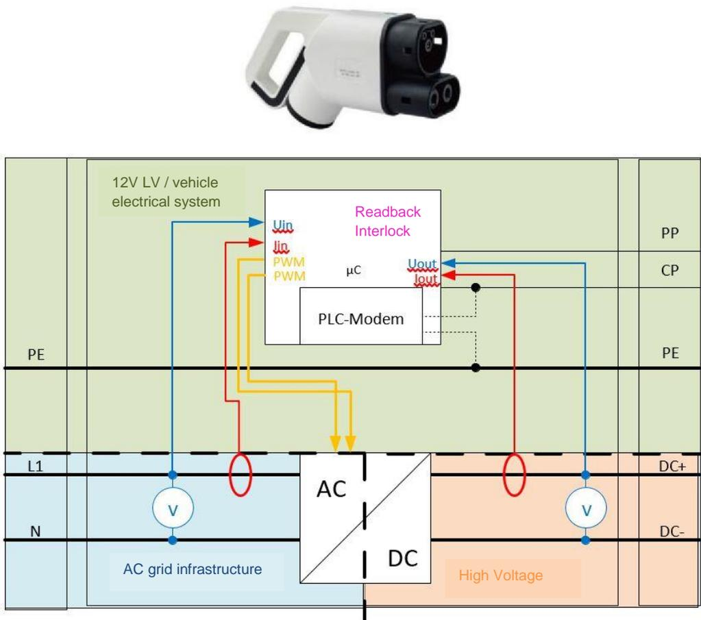
**Figure 5: Block Diagram Power Plug Charger / Plug Power Supply**
