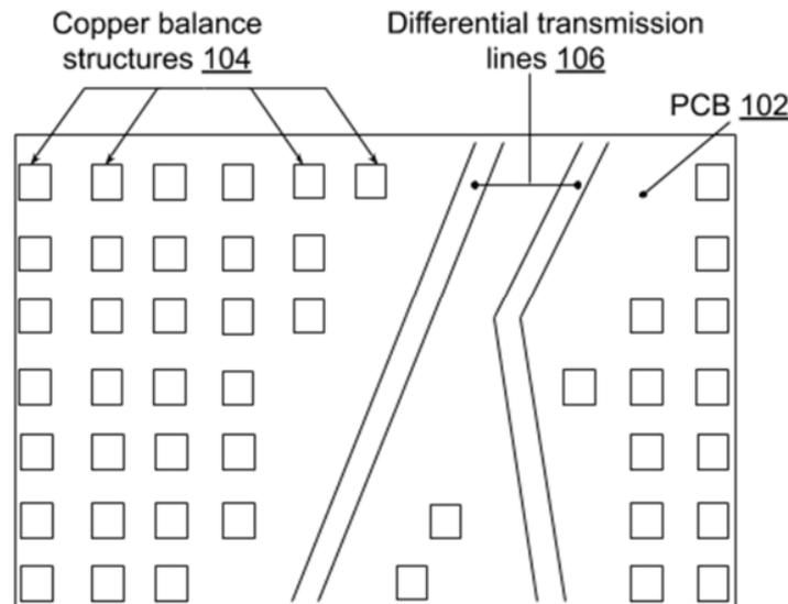
**Fig. 1: Copper balance structures in printed circuit boards**
