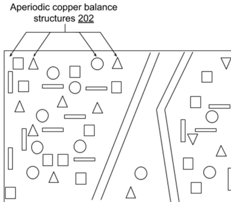
**Fig. 2: Aperiodic structures used for copper balance in PCBs**
