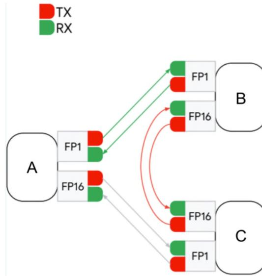
**Fig. 2: Pairwise interconnect of fiber-optic pairs within a branching unit**
