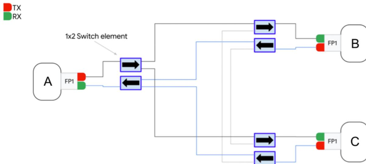
**Fig. 4: An alternative implementation of fiber-optic interconnects within a branching unit**
