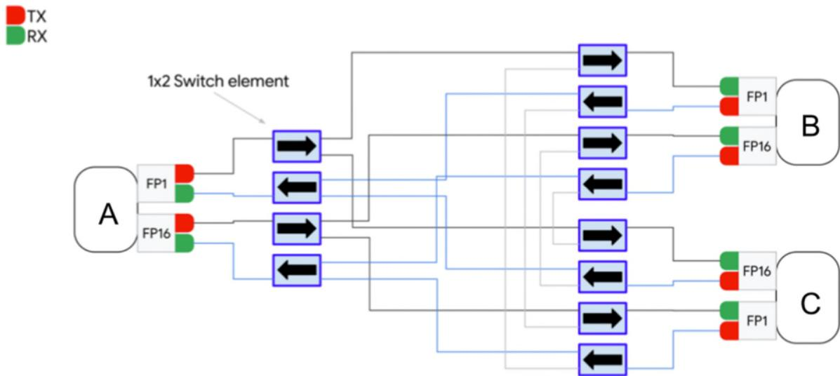
**Fig. 3: An example implementation of pairwise interconnect of fiber-optic pairs within a branching unit**
