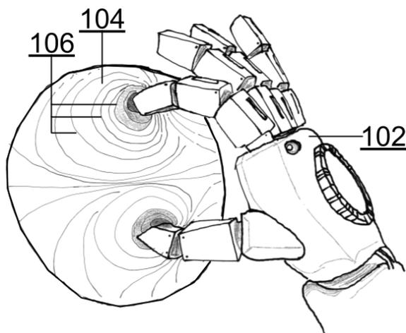
**Fig. 1: Strain contour pattern on an object being picked up**
