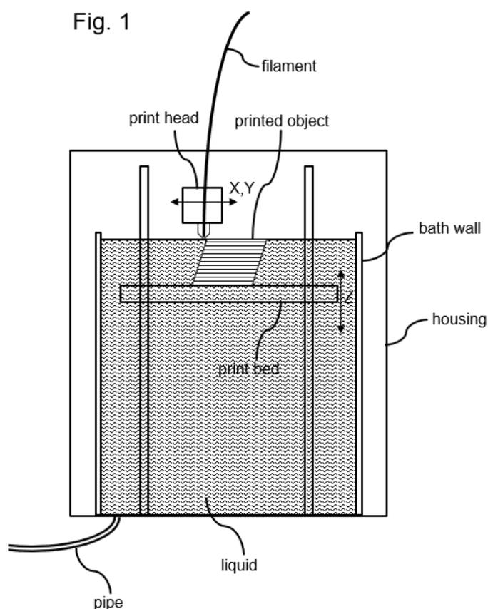
Figure 1 shows a schematic side view of a first example of the FFF printer with a print bed that can be moved up and down in the Z-direction. A print head can be moved in the X and Y directions by means of a gantry which is not shown here. In the example shown in Figure 1, the bath envelops the build platform (i.e. the print bed) in all its freedom of motion.
