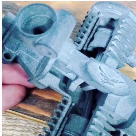
Figure 2. Example of a complex assembly with several inner moving parts working according to a gear manually powered.
