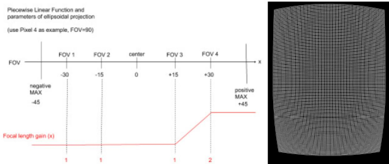
**Figure 4: Piecewise axis tuning curve and resultant ellipsoidal projection.**
