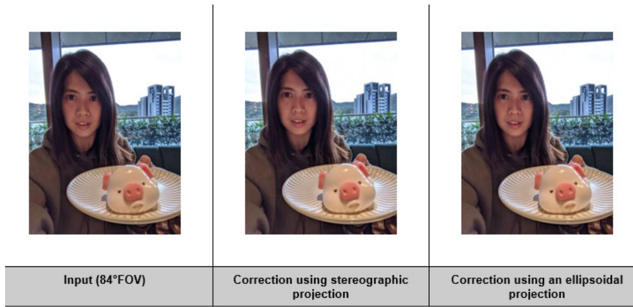
**Figure 6: Uncorrected image, an image with distortion correction using a stereographic projection, and an image with distortion correction using an ellipsoidal projection.**
