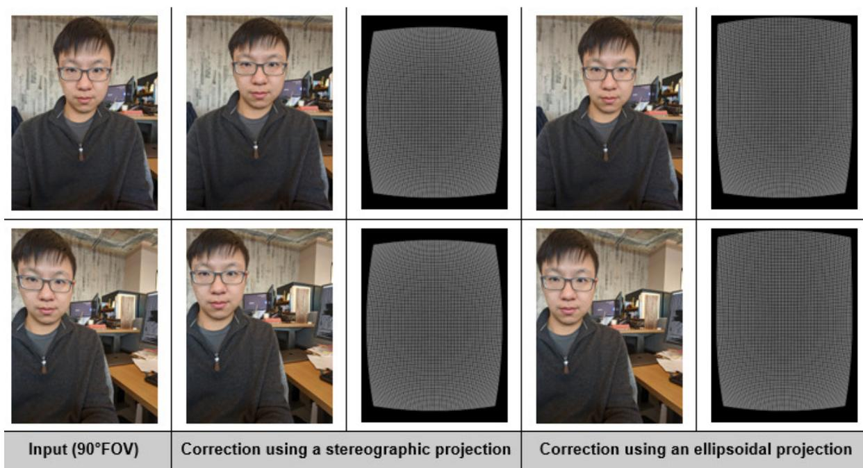
**Figure 5: Uncorrected images, images with distortion correction using a stereographic projection, and images with distortion correction using an ellipsoidal projection.**
