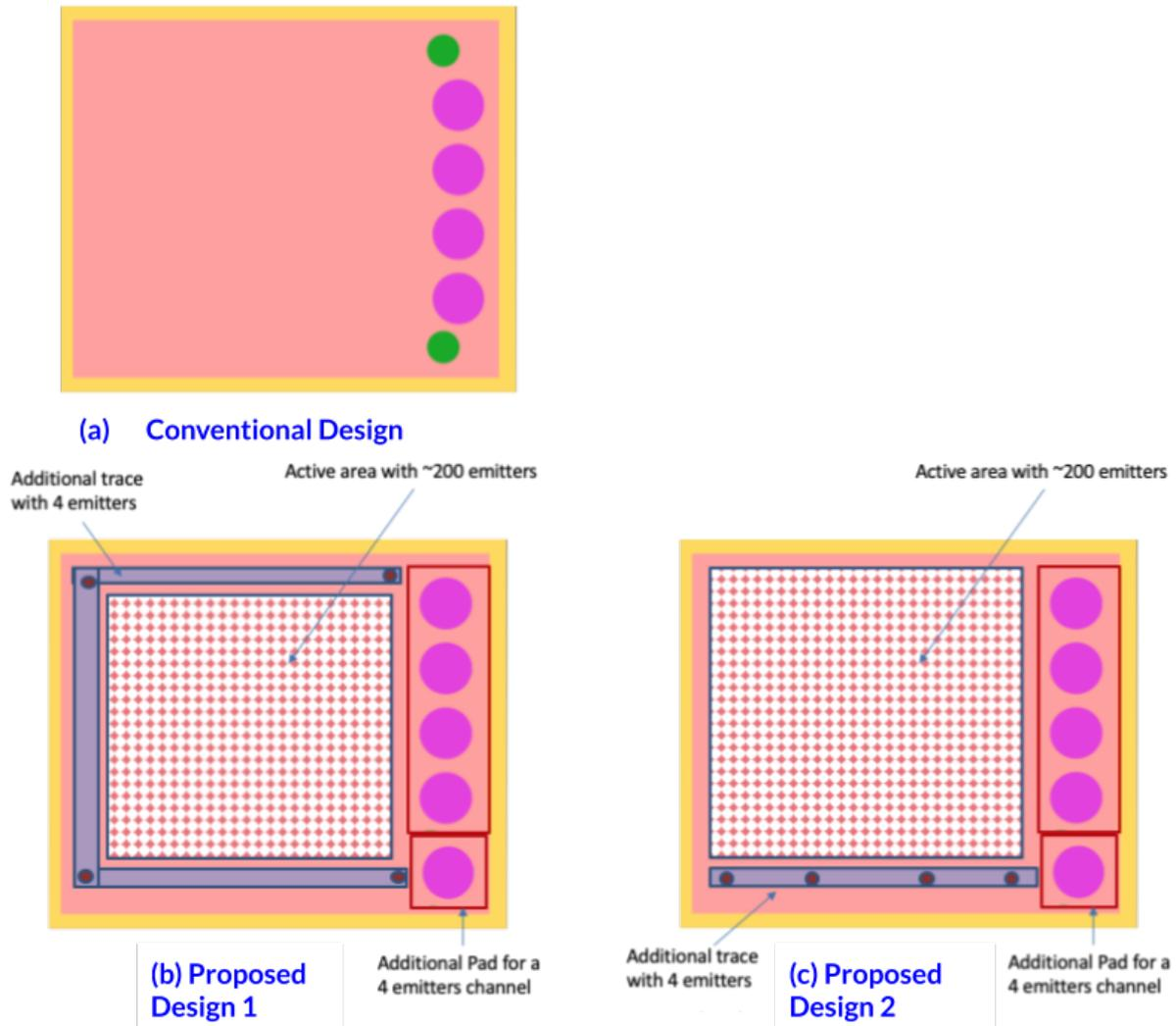
**Fig. 2: VCSEL chip: (a) Conventional design; (b) Proposed design with dedicated channel (option 1); (c) Proposed design with dedicated channel (option 2)**
