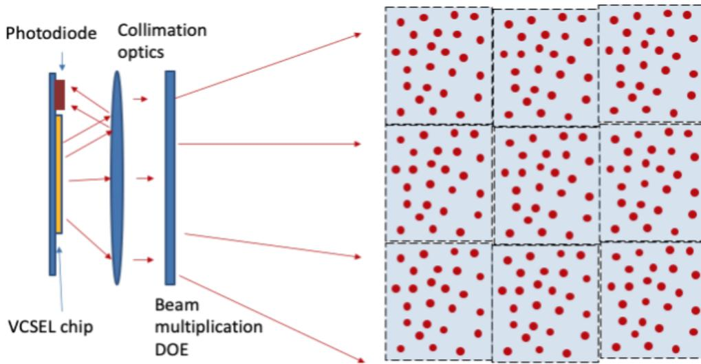
**Fig. 1: Projector with VCSEL chip**
