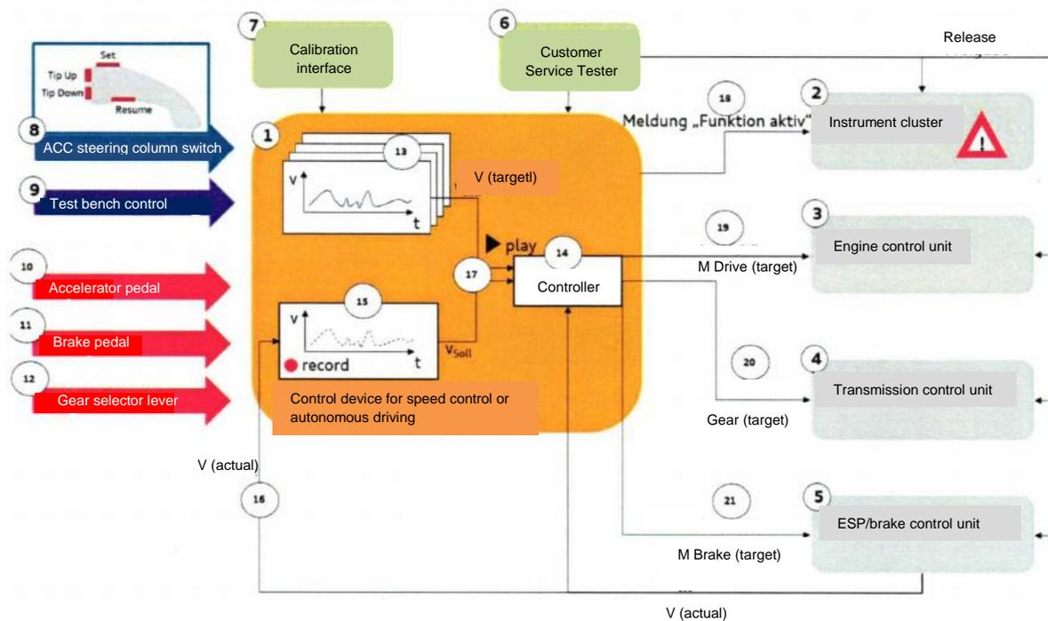
**Figure 1: Control unit architecture, signal flows**
