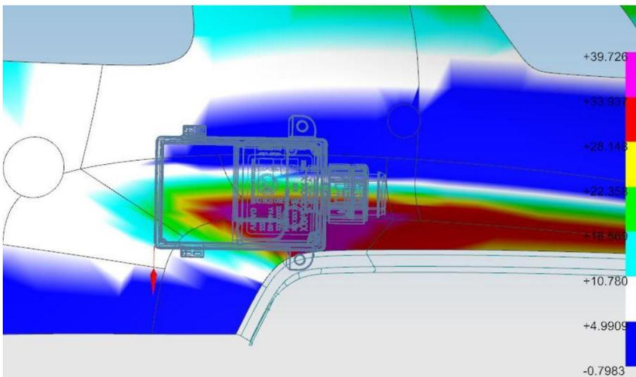
**Figure 3: Search for the optimum installation position only within the favourable curvature range**
