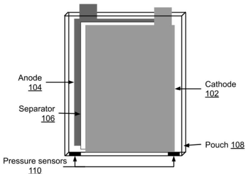
**Fig. 1: Battery pack with integrated pressure sensors**
