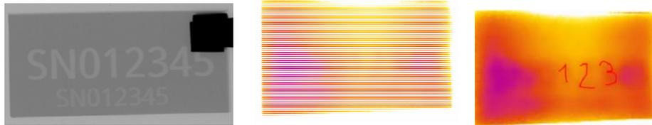
Figure 2: The metainformation (SN012345) can be read using a Thermal Camera when the part is subject to a thermal gradient
