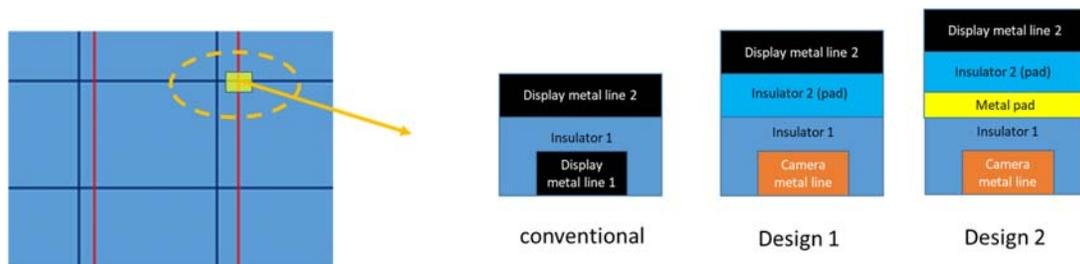
**Figure 1.** Structure of integrating camera and display signal lines.
