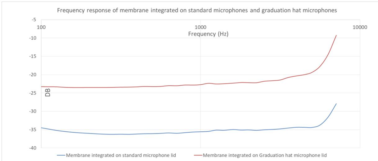
Figure 4: Frequency response comparison between membrane integration on standard microphone lid and Graduation Hat lid.
