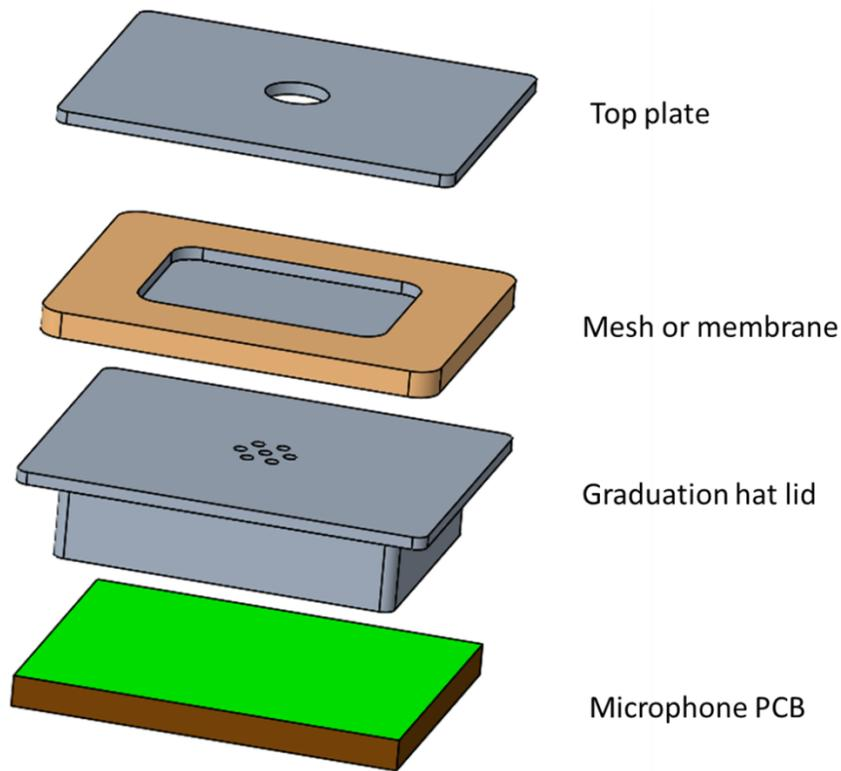
Figure2: Example of Graduation Hat design on microphones
