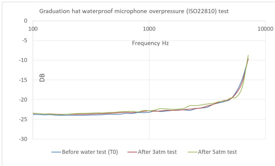
Figure 5: 3/5atm waterproof performance of Graduation Hat microphones
