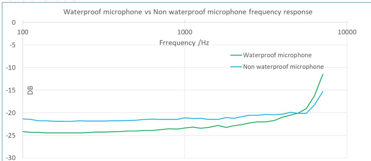
Figure 3: Frequency response comparison between Graduation Hat waterproof and non-waterproof microphones.
