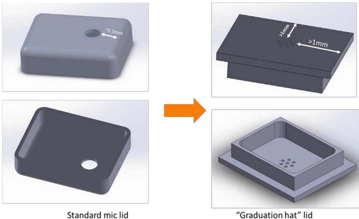
Figure1: Example of Graduation Hat design drawings
