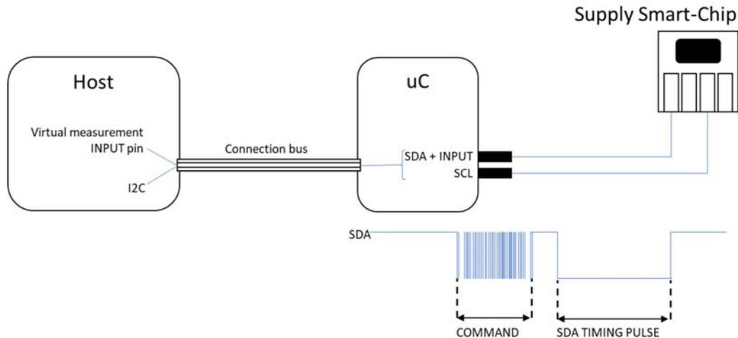
Figure 1 - Solution based on "virtual" measurement input pin
