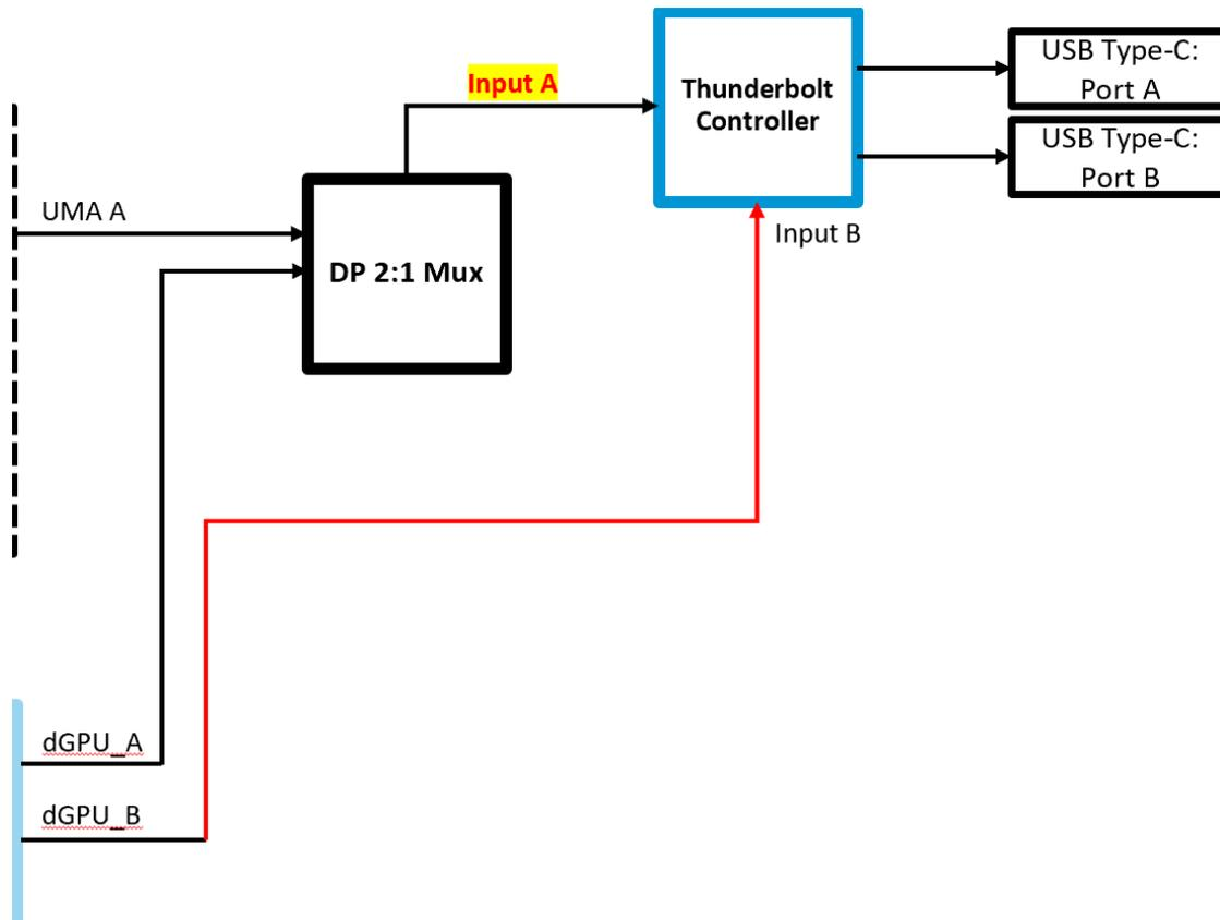
**Figure 2: One less multiplexer design to enable docked pre-boot external display support**
