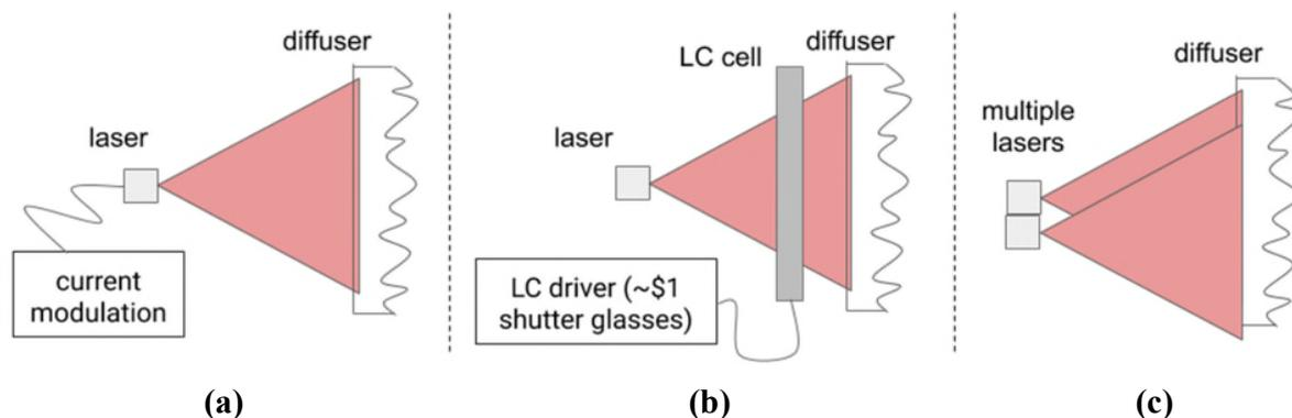
**Fig. 4: Generating a time-varying speckle pattern**
