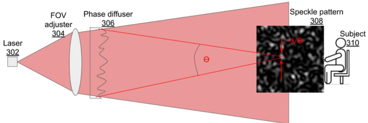
**Fig. 3: Dot projector based on phase diffuser**
