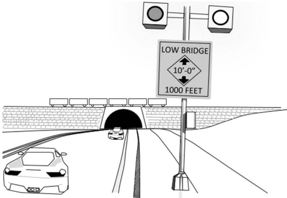
**Fig. 2: An example of a warning sign for insufficient vertical clearance**
