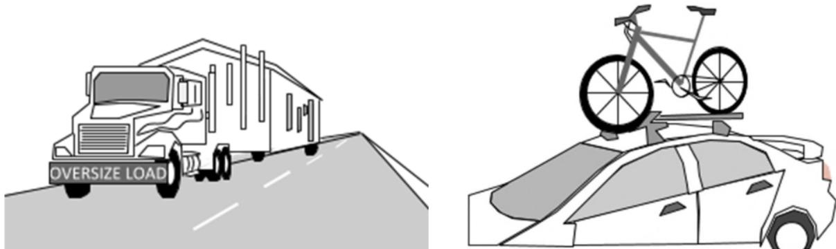
**Fig. 1: Vehicles with variable dimensions**
