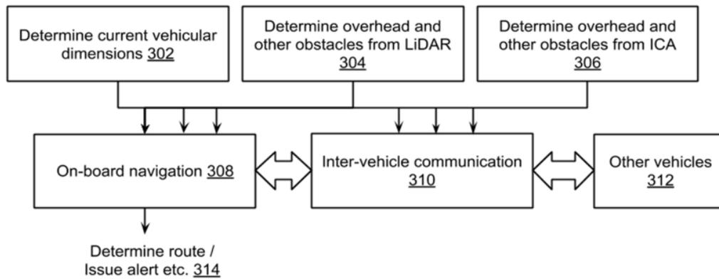
**Fig. 3: Overhead collision alerts and navigation planning**
