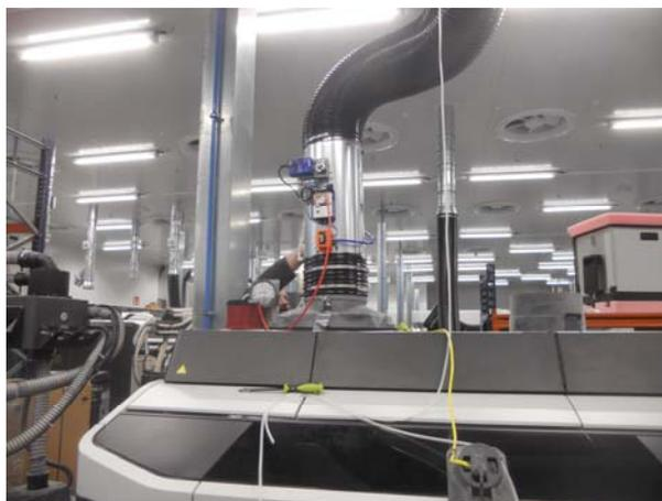
The objective pressure is mainly determined in such a way that the 3D Printing Machine operates in a similar way as working without Extraction System. In theory, could be set to a gauge pressure of  $0$  Pa, but in general some negative value is preferred to avoid local gauge pressures above  $0$  Pa which will lead to leaks towards the room.
