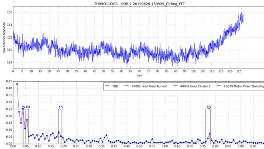
Figure 4: Sample Evaluation Plot. Used to correlate Specific Frequencies with Gear Train Components that cause Banding.
