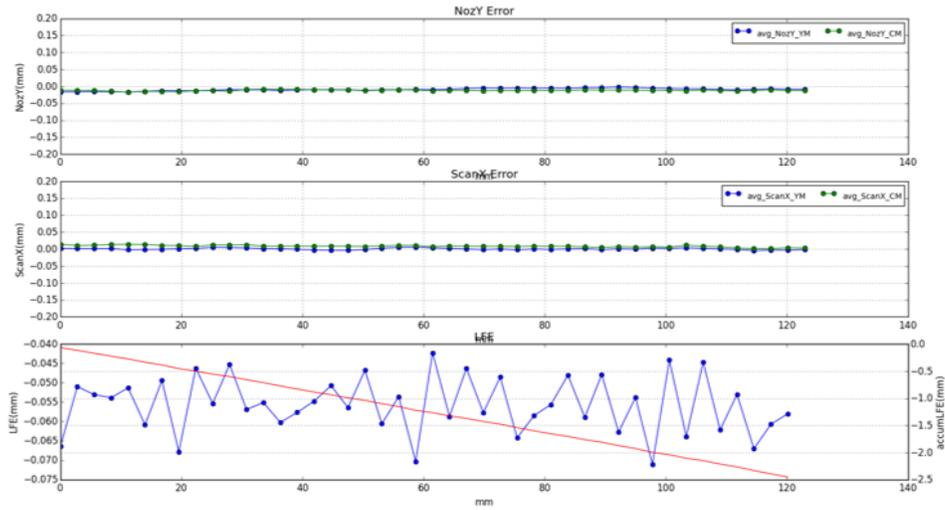
Figure 3: Sample Evaluation Plot: Measures Color Registration and Image Length. Misregistration is attributed to Defective Rollers; Image Length Variation can be compensated for using a FW Constant.
