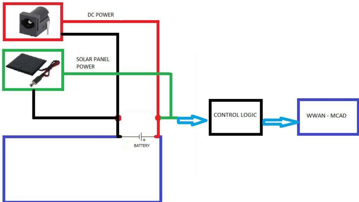
**Figure 2: Illustrates a simple implementation for IoT Mode using a small integrated solar array.**
