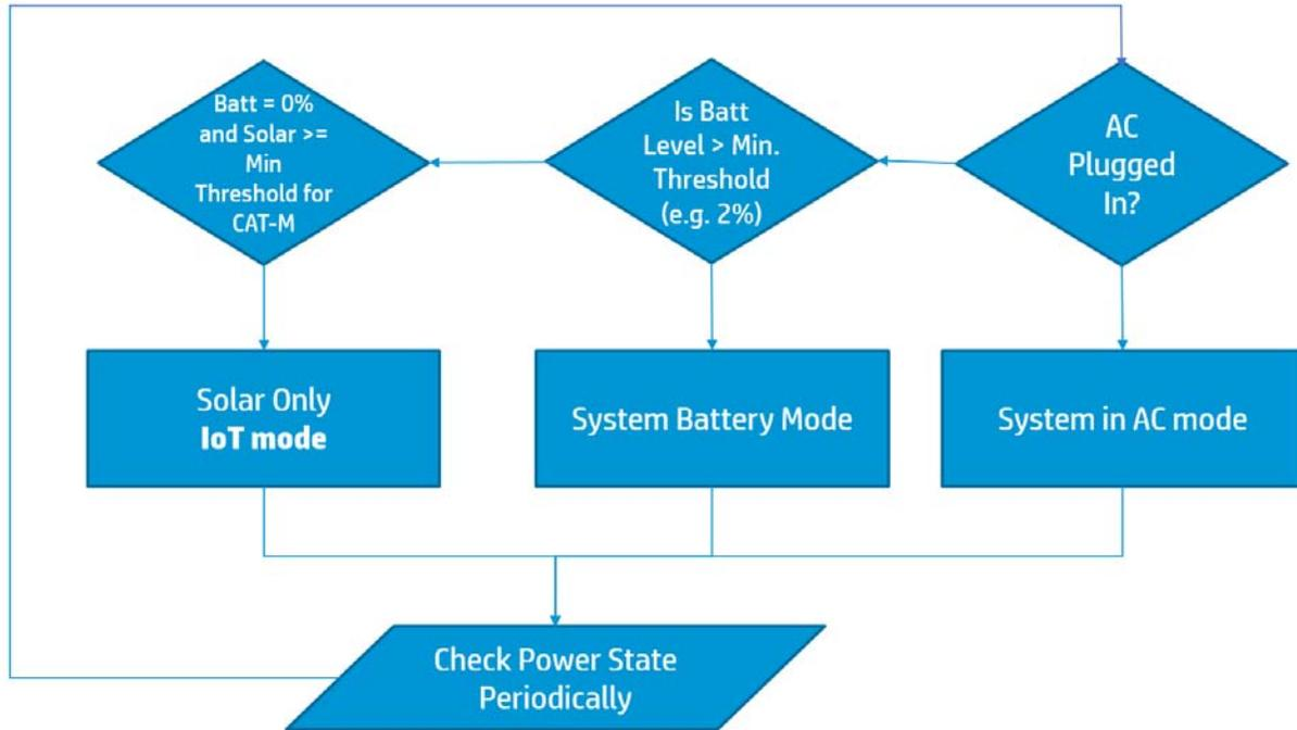
**Figure 1: Flowchart of the various system power states including IoT mode.**
