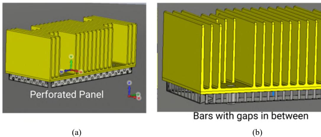
**Fig. 5: EMI-suppression structures with provision for enhanced airflow**
