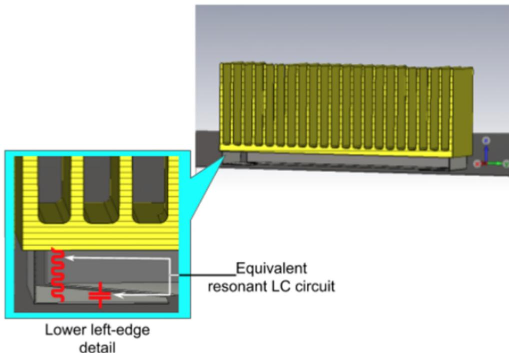
**Fig. 2: Heat sink geometry that reduces EMI**
