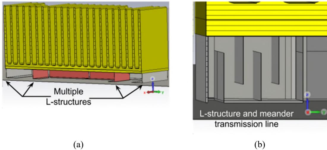
**Fig. 4: Examples of EMI-suppression structures (a) multiple L-structures (b) L-structure and meander transmission line**
