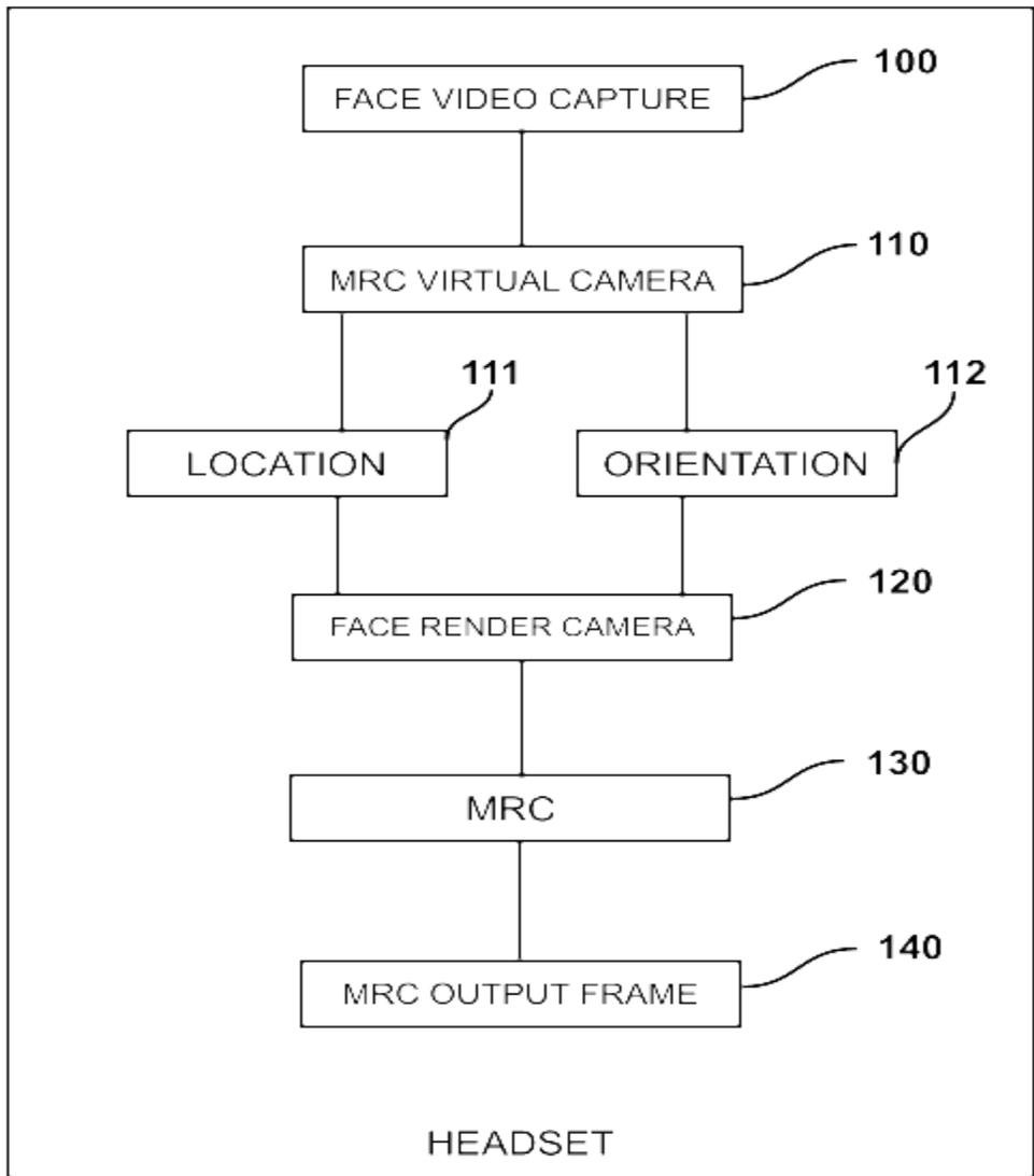
Figure 3: The process flow of the MRC system
