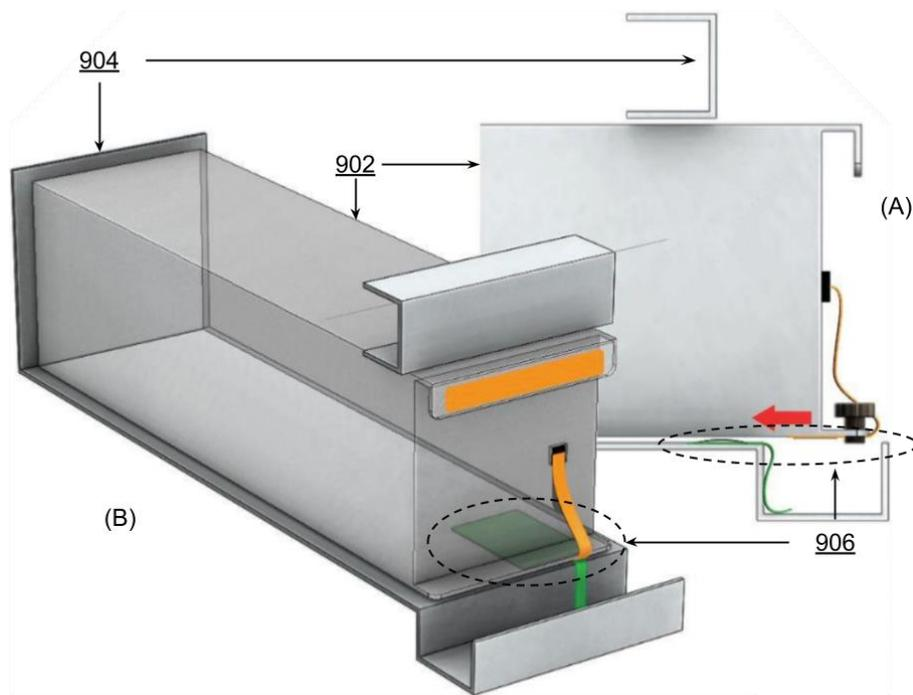
**Fig. 9: (A) Side view and (B) perspective view of equipment being inserted into a rack**
