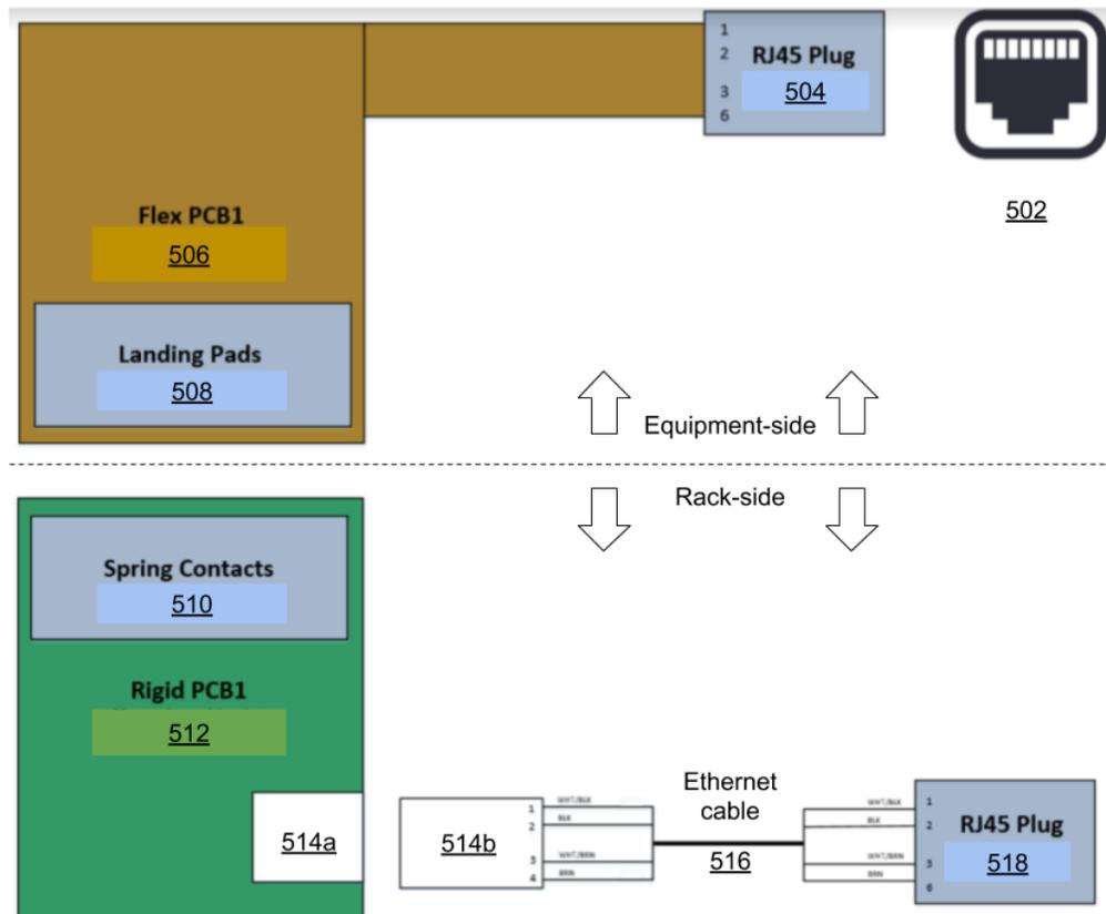
**Fig. 5: Electrical schematic of the springboard adapter**
