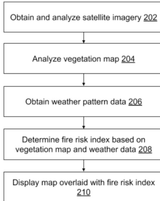
**Fig. 2: Determination of fire index data from satellite and weather data**
