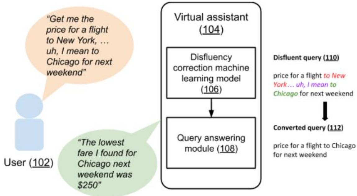
**Fig. 1: Correction of a disfluent query using a machine learned model**
