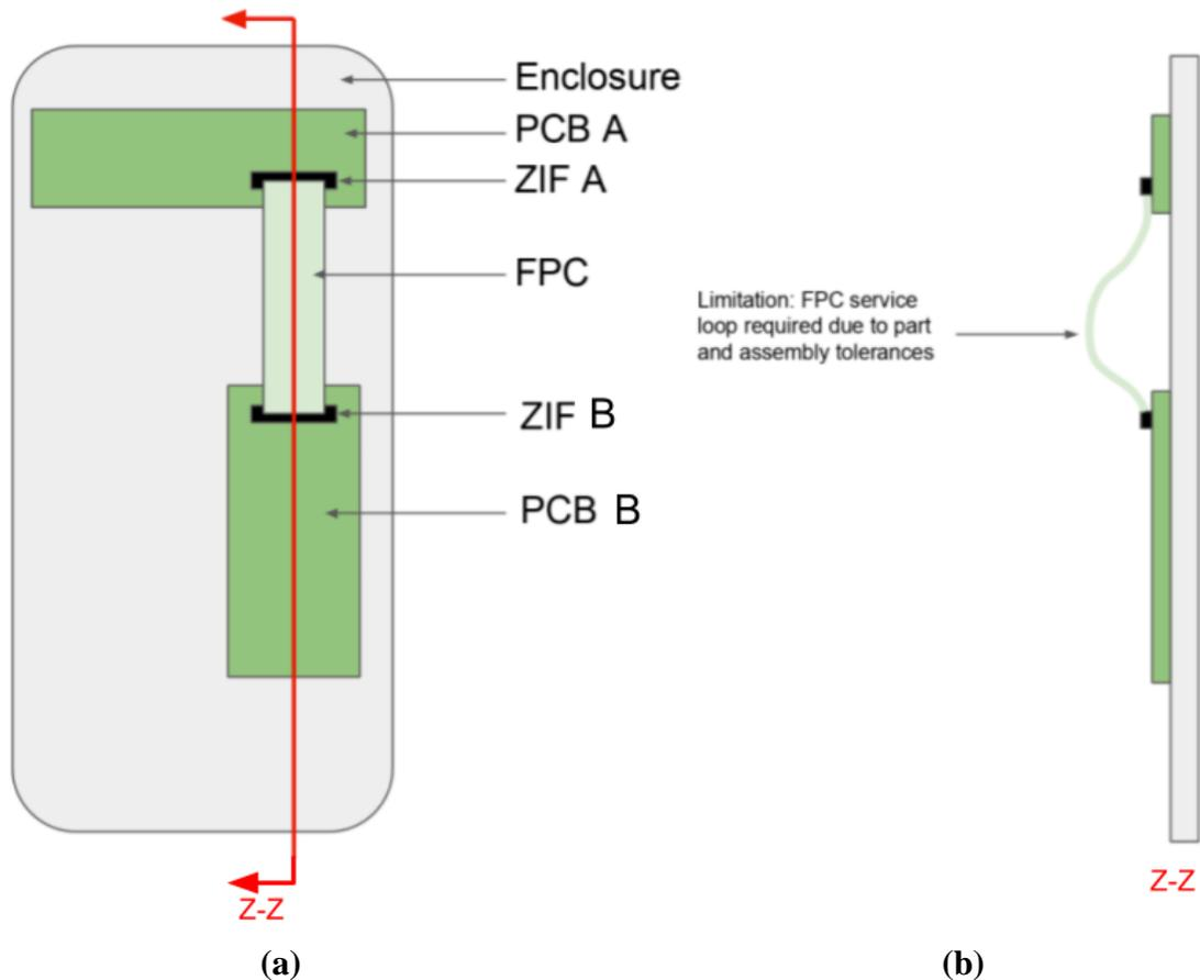
**Fig. 2: An FPC connecting two PCBs: (a) Top view; (b) Cross-section at ZZ. Due to part and assembly tolerances, a service loop forms in the FPC**
