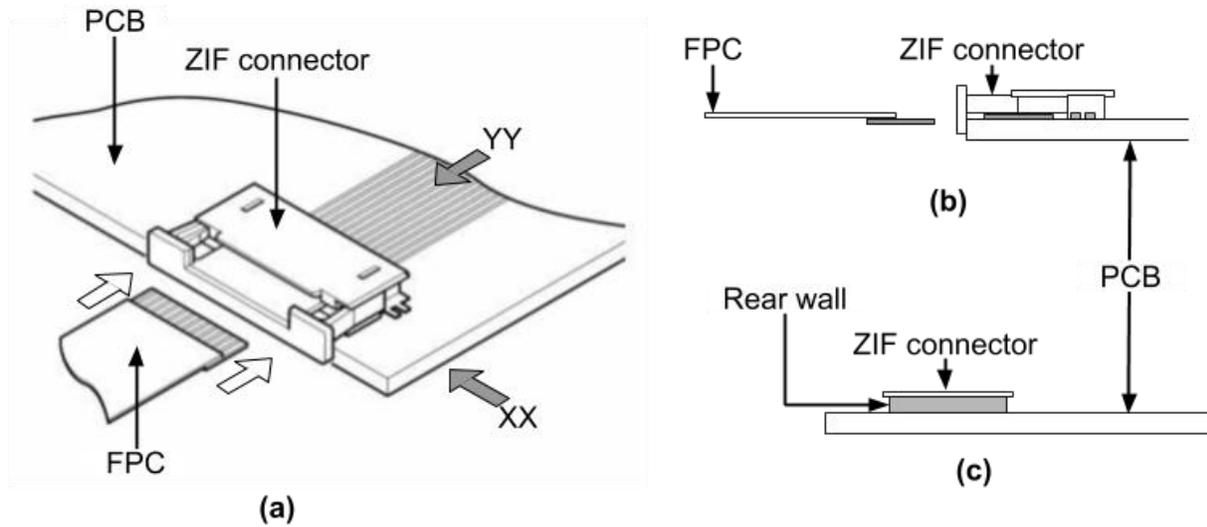
**Fig. 1: ZIF connector: (a) Perspective view; (b) Side view (from XX); (c) Rear view (from YY)**
