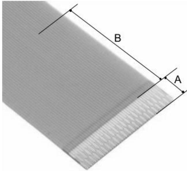
**Fig. 4: Parts of an FPC**
