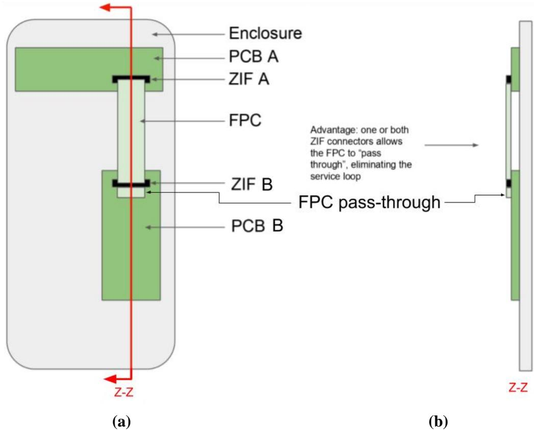
**Fig. 3: Eliminating the service loop of an FPC: (a) Top view; (b) Sectional view at ZZ, illustrating the passing through of the FPC at ZIF connector B**
