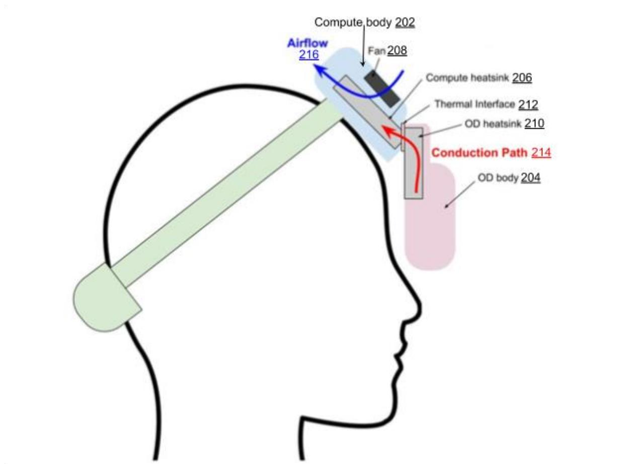
**Fig. 2: Conductive coupling between constituent modules (active mode)**
