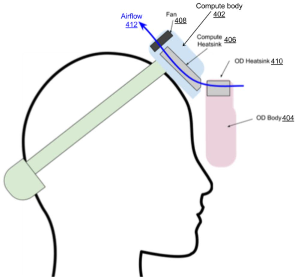
**Fig. 4: Convective coupling between constituent modules (active mode)**
