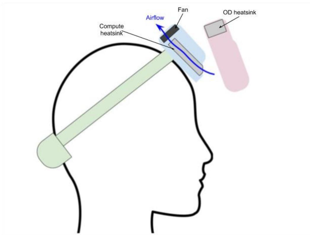
**Fig. 5: Convective coupling between constituent modules (standby mode)**
