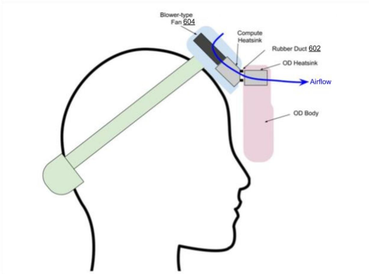
**Fig. 6: An example implementation of convective coupling**
