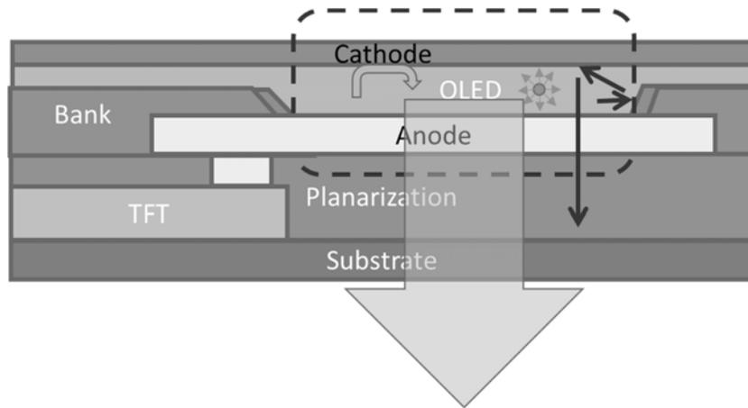
**Figure 2.** Cross session of proposed bottom emission OLED structure.
