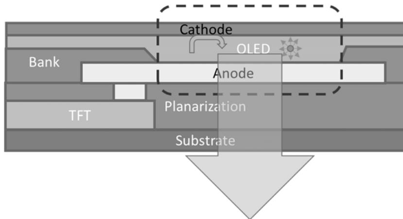
**Figure 1.** Cross section of conventional bottom emission OLED structure.
