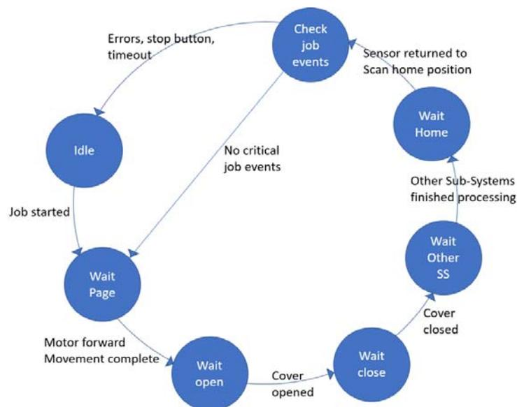
Figure 2: Overall system state diagram
