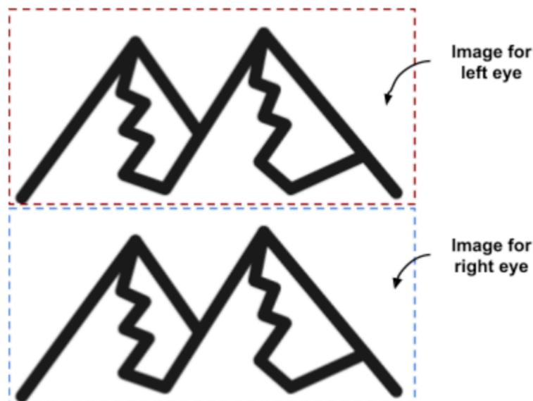
**Fig. 2: Stereoscopic video - over-under configuration**
