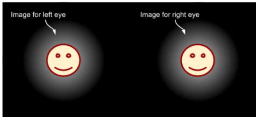
**Fig. 1: Stereoscopic video - side-by-side configuration**
