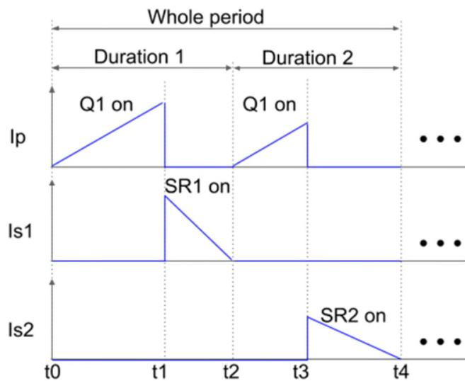
**Fig. 4: Control waveforms for critical conduction mode**
