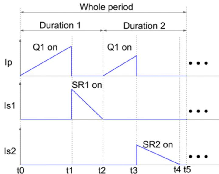
**Fig. 5: Control waveforms for combined DCM-CRM mode**
