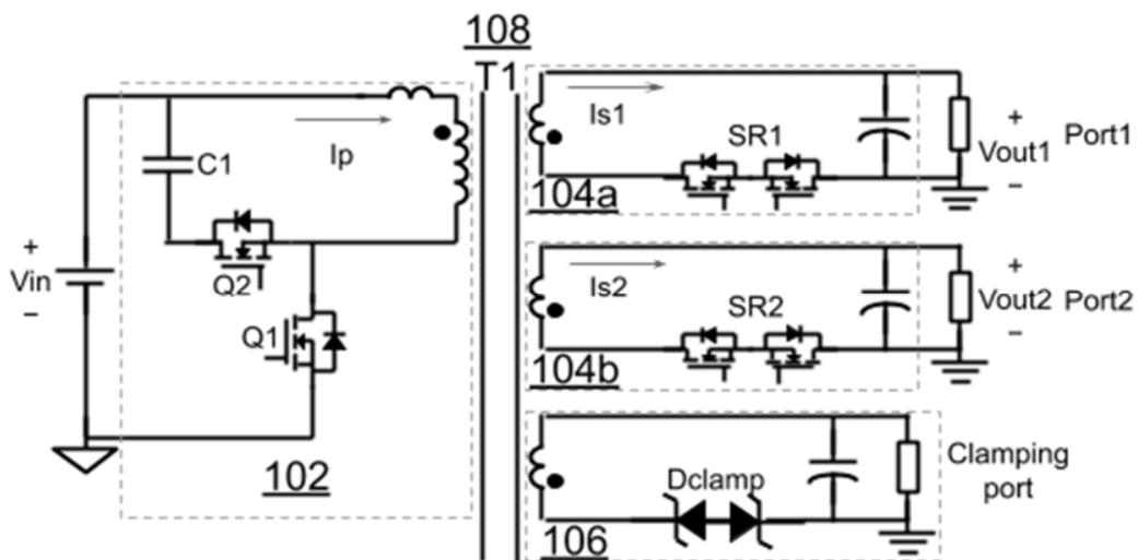
**Fig. 2: Circuit schematic of a multi-output DC-DC converter**
