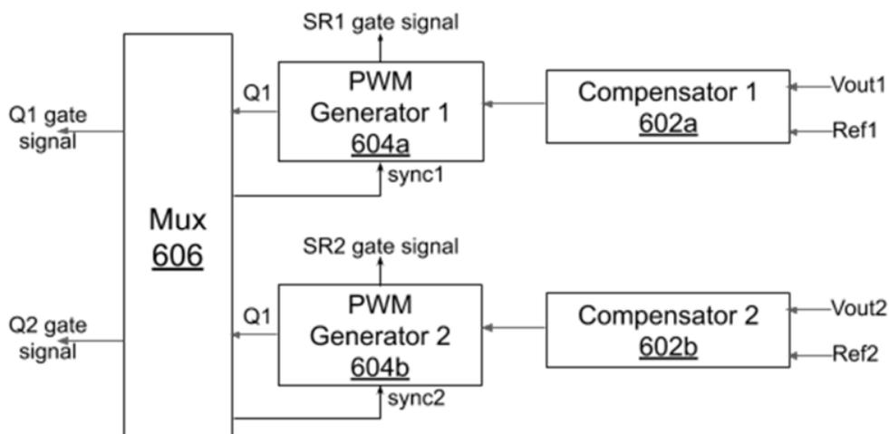
**Fig. 6: Control-signal generator circuit**
