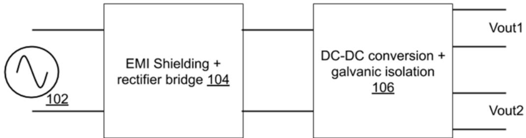
**Fig. 1: Block diagram of a multi-output power adapter**
