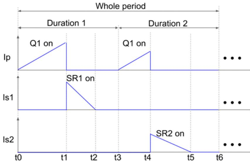
**Fig. 3: Control waveforms for discontinuous control mode**
