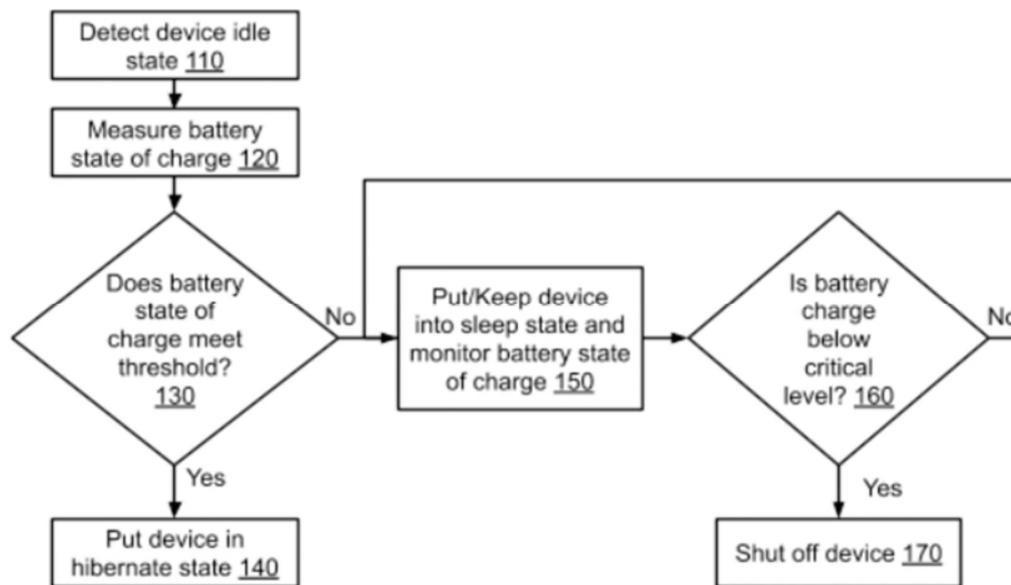
**Fig. 1: A low power state is selected based on a battery state of charge**
