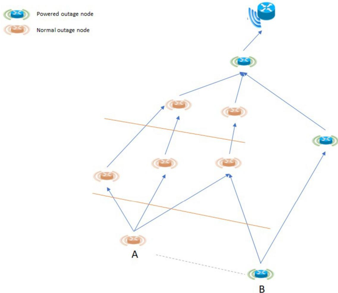
Consider for the example of Figure 1 that each node is experiencing an outage. In this example, Node A cannot forward a PON message to the outage server because none of its parent nodes has a power capability when the outage occurs. However, there is Node B, which help could forward the PON message, yet it cannot be chosen as a Routing Protocol for LLN (RPL) parent because of higher rank. Finding a reliable parent could greatly increase the PON success rate when a nested outage occurs.
