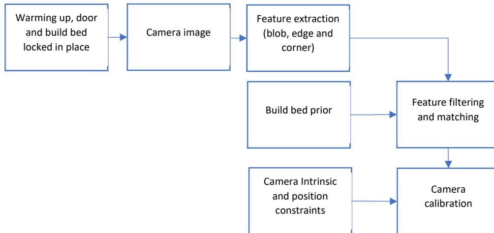
*Figure 2: Block diagram of the autocalibration of the camera*
