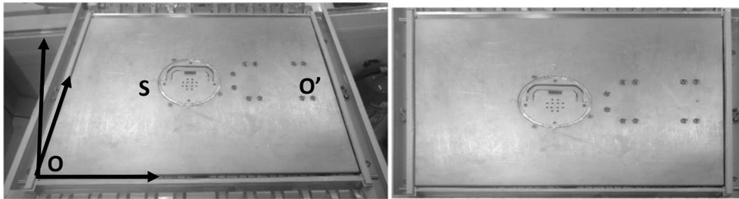
*Figure 1: Left: Setup of the system with the Build Surface  $S$ , the camera  $C$  and the world origin of coordinates  $O$  (solid axes) and the camera origin of coordinates (dashed axes). Right: Flattened image of the build area.*
