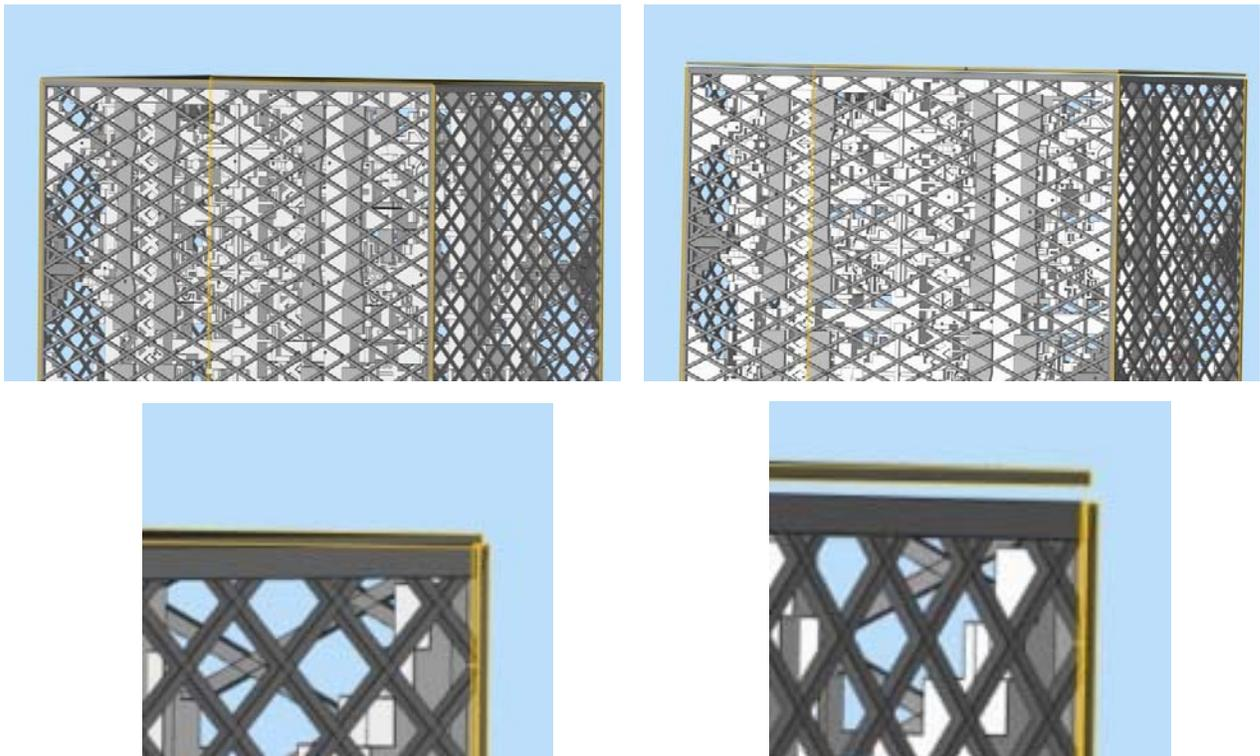
*Figure 1: On the left, the old build envelope for the external cooling. On the right, the new build envelope design with the separation of the top cover.*
