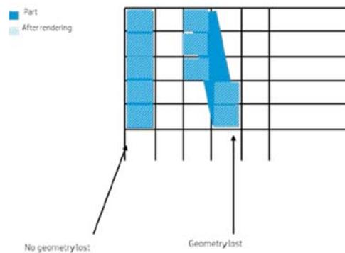
Figure 2: Difference between rendering a rectangle parallel to printing axes (left) vs one tilt (right)
