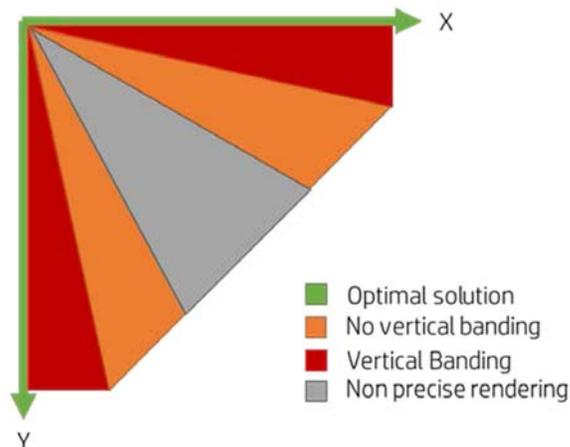
Figure 5: Surface orientation vs render accuracy and vertical banding defects
