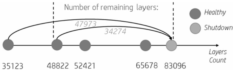
Figure 2 - Calculating the Remaining layer target before a shutdown
