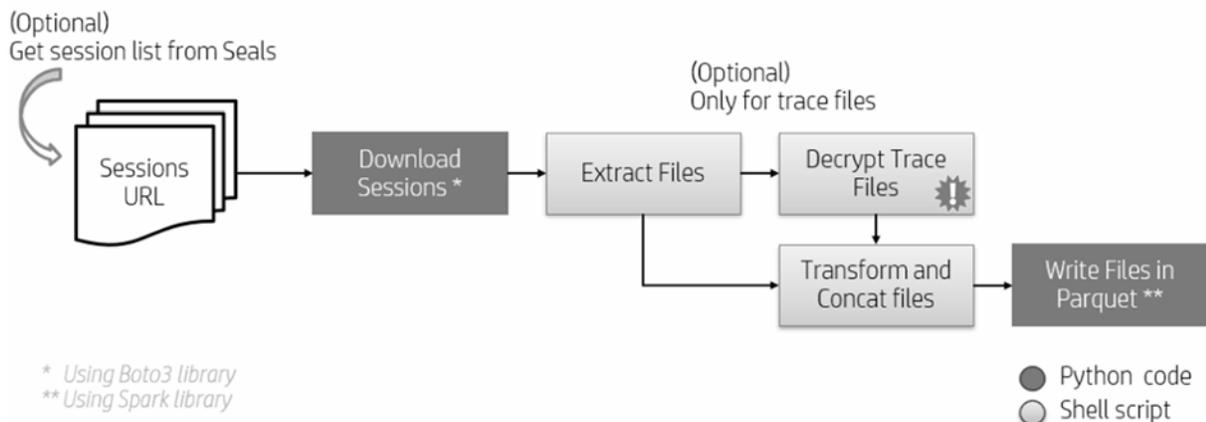
Figure 1 - Data ingestion workflow
