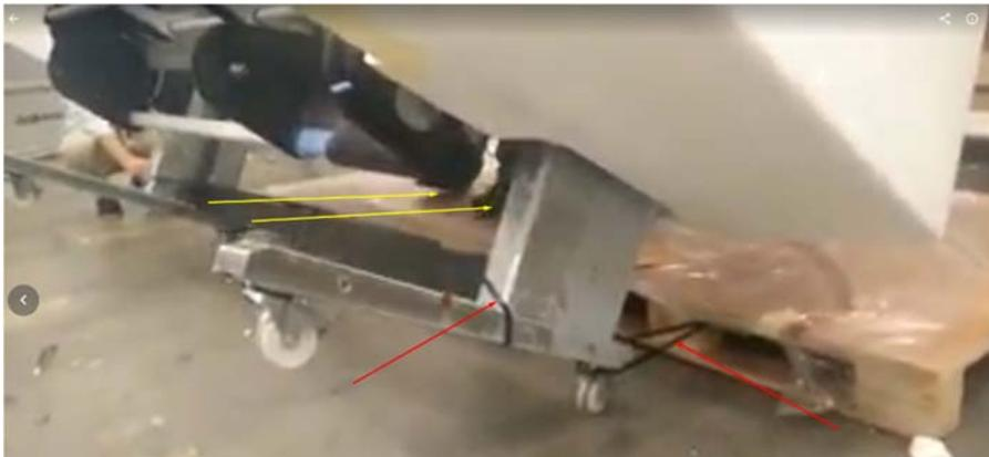
Figure 4: still image while lifting the machine. The red arrows show the strip in tension, working against the natural runaway of the machine. Yellow arrows show the position of the feet of the operators, acting as “weight” to counter-rest the machine weight.
