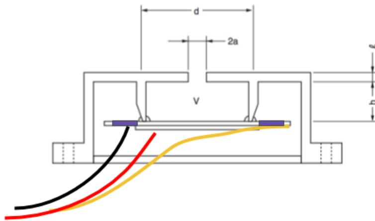
**Fig. 4: Placement of the slotted antenna within a nodal-supported piezo buzzer**
