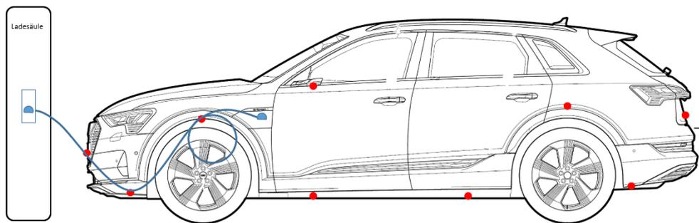
**Figure 4:** Cable routing over vehicle mounting points with cable loop to charging facility
