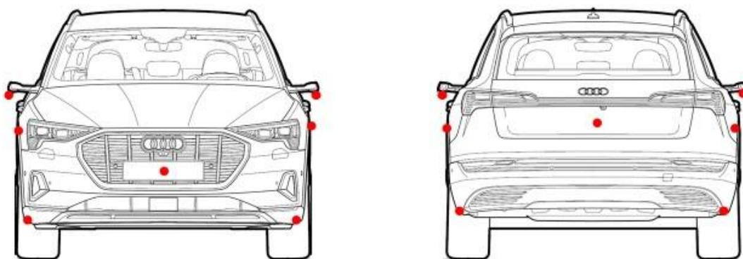
Figure 2: Possible locations for vehicle charging cable attachment points
