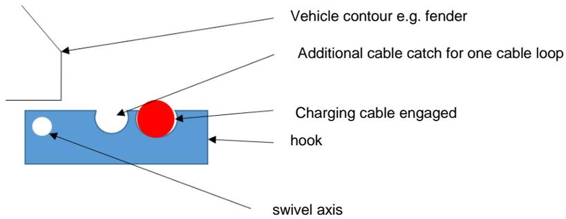
**Figure 3:** Simplified hook geometry of the vehicle attachment points for the charging cable
