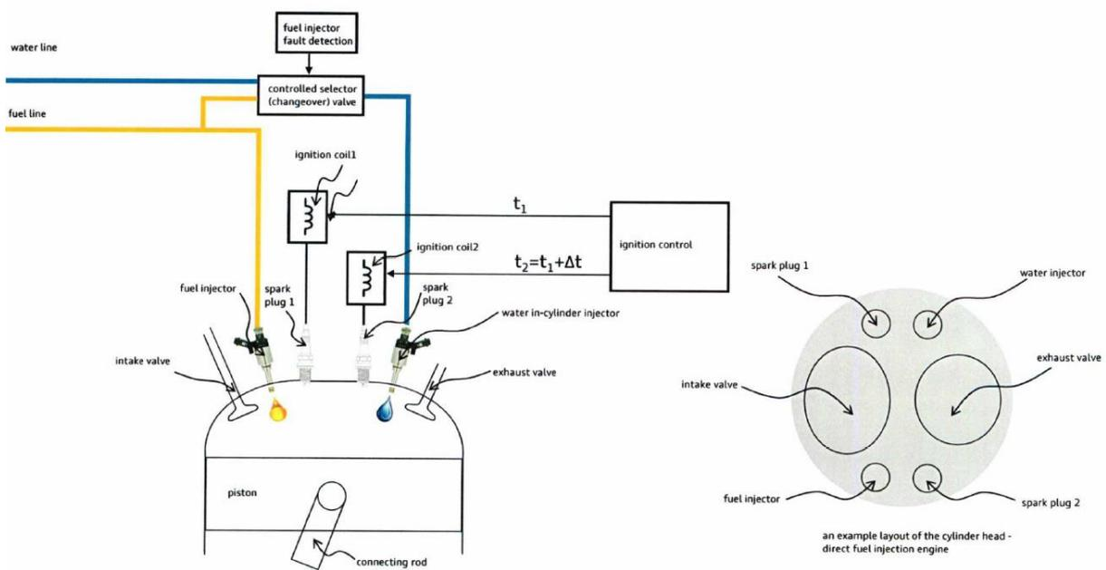
Figure 3: Direct fuel injection engine
