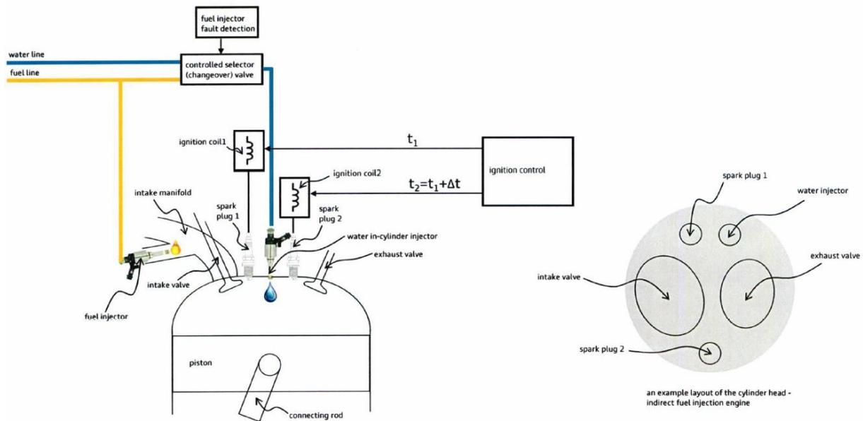
Figure 2: Indirect fuel injection engine
