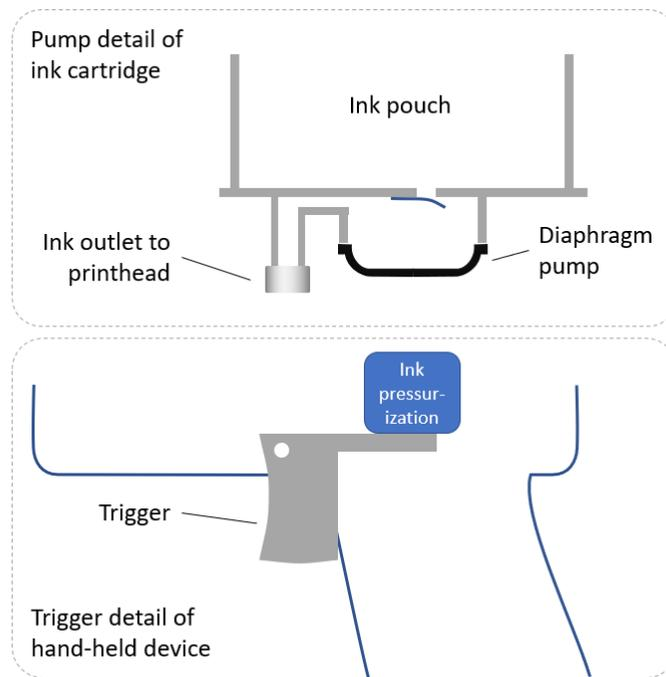
Figure 3. The key elements of the single use printhead ink cartridge above the mating features of a hand-held device
