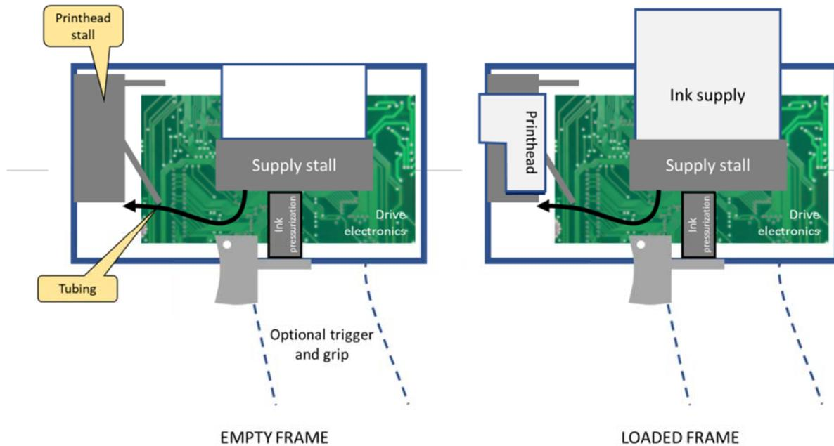
Figure 2. Component architecture of a compact coder
