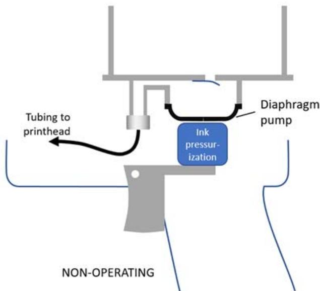
Figure 4. Mechanical linkage between the trigger of the hand-held device and the diaphragm pump of the ink cartridge
