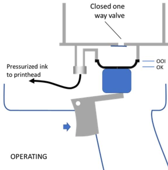
Figure 5. Actuator pushed up against the diaphragm pump by the trigger.
