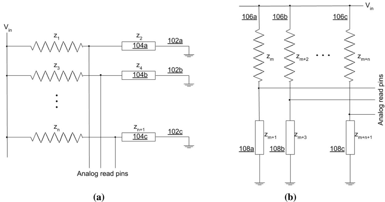
**Fig. 1: Resistive grid to detect and localize damage**
