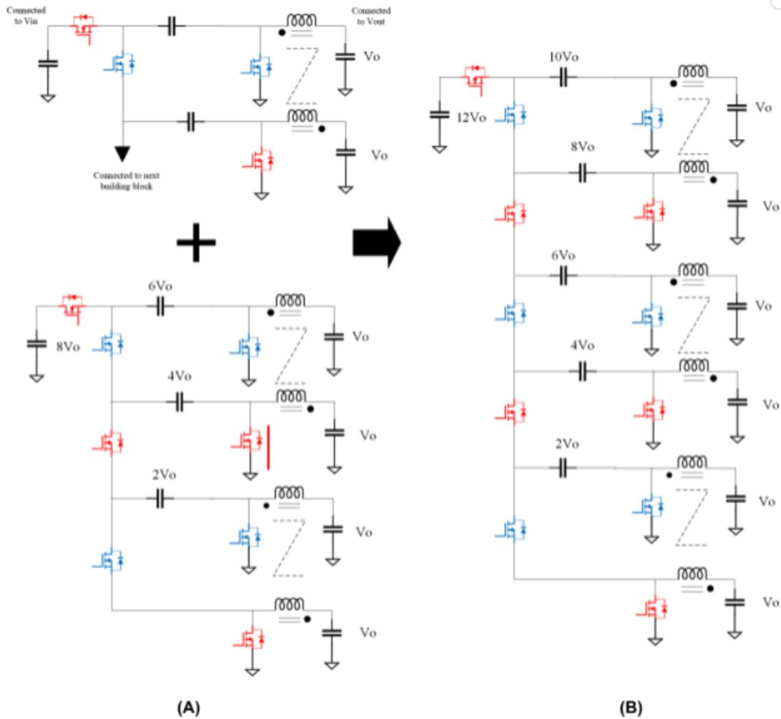
**Fig. 6: A 12:1 DC-DC converter (A) Construction from modular building blocks (B) A 12:1 DC-DC converter**
