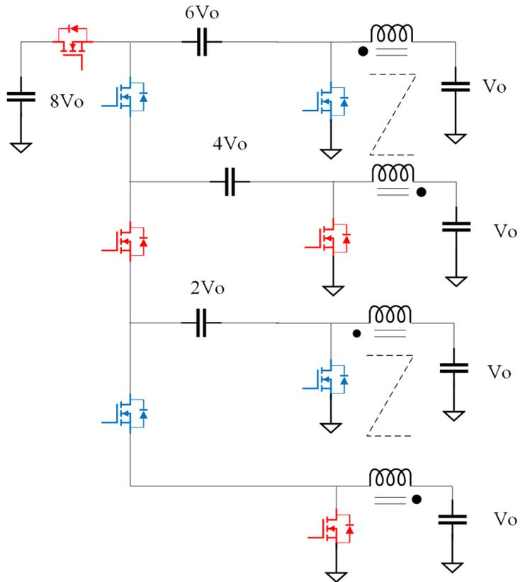
**Fig. 4: An 8:1 DC-DC converter**
