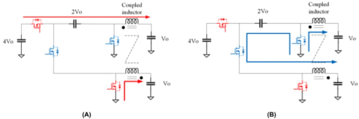
**Fig. 3: Operating stages of a 4:1 DC-DC converter (A) Stage-1 - the red switches are closed and the blue switches are open (B) Stage-2 - the red switches are open and the blue switches are closed.**
