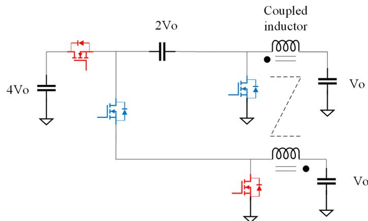
**Fig. 2: A 4:1 DC-DC converter**
