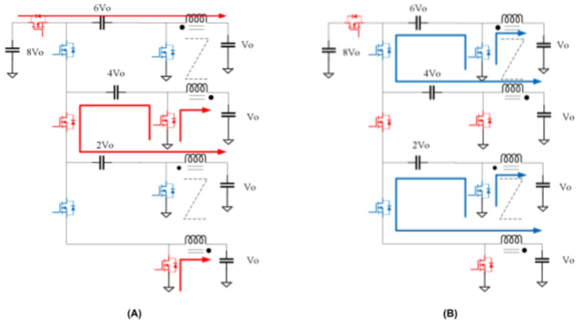
**Fig. 5: The operating stages of an 8:1 DC-DC converter (A) Stage-1 (B) Stage-2**
