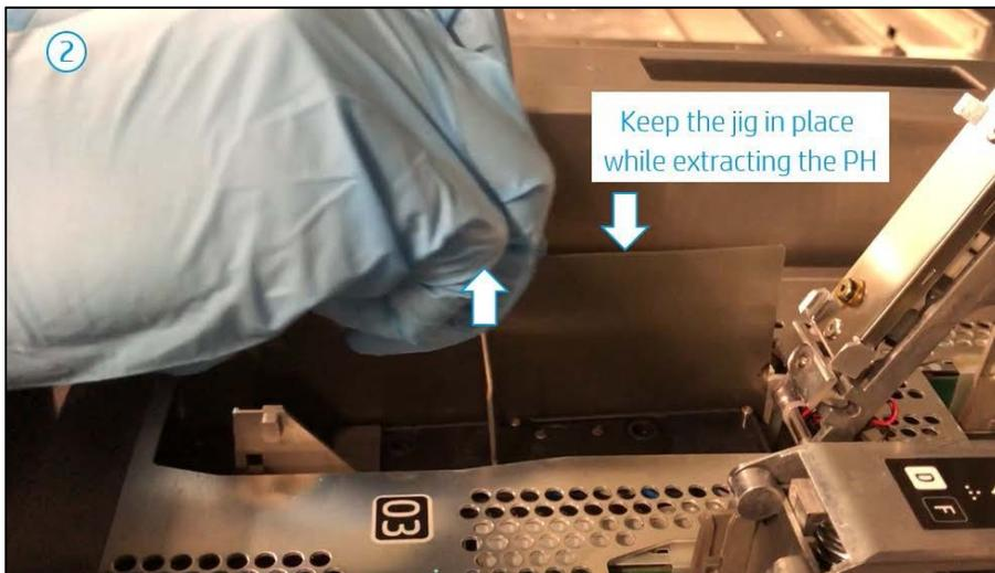
Figure 3 – Step 2 in the process of replacing the print head using the new tool
