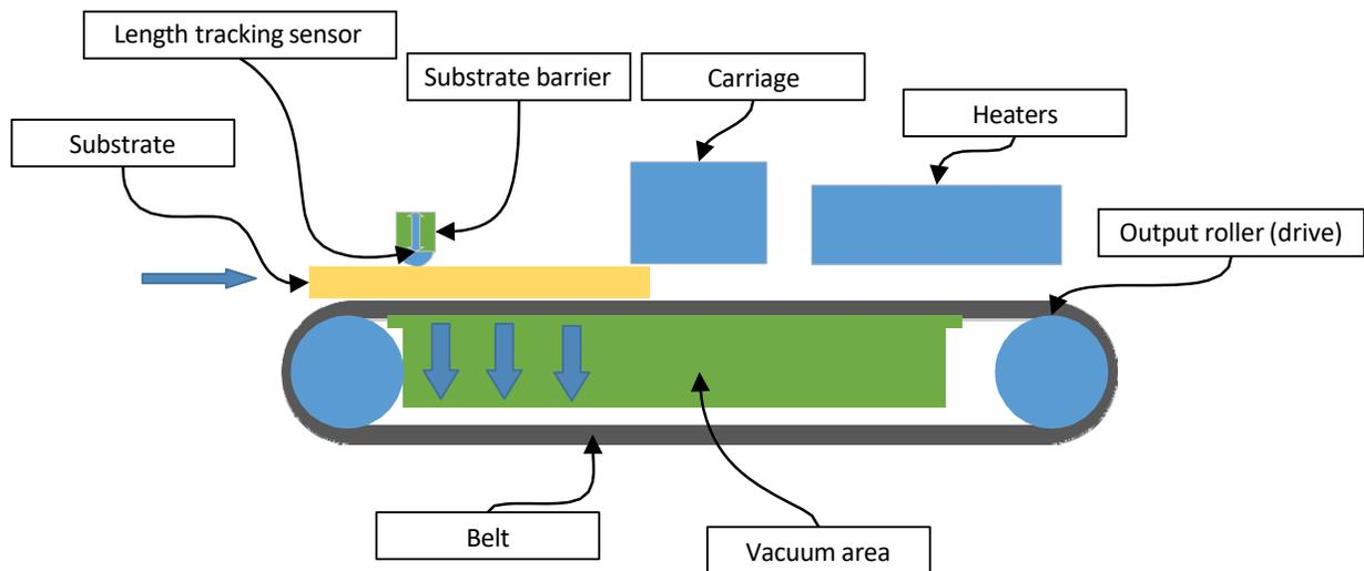
In the entrance of the belt usually there is a substrate barrier that can moves up and down. This barrier is used, among other uses, to avoid substrate with non-negligible thickness placed over the input area of the belt to enter to the printing zone before the printer is not ready for print it.
