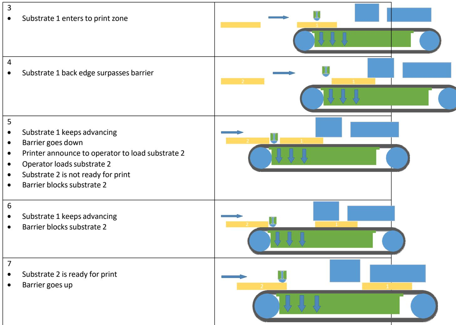
In the step 4 the length of the substrate is needed to know when the barrier can be moved down. Knowing the exact length is critical to do this operation just in time, and not before or after. If the barrier is moved down before the substrate surpasses the barrier, the barrier will crash with the substrate; if it's moved down much after, it's a loss in throughput.
