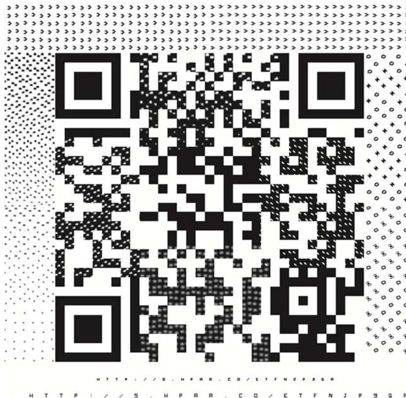
Fig. 2: QR code image with an embedded security ID and embedded public key features
